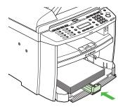
Adjust the paper guide rail to match the size of
